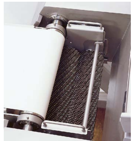
A conveyor drops product into the tenderizer rollers.
